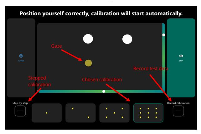
Before a calibration is started, it is possible to select how many points are to be used for the calibration. A higher number of points takes longer, but usually achieves more accurate results.
